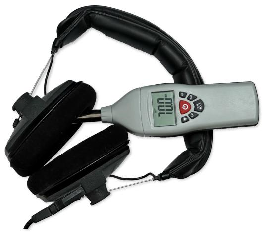
Position the dB meter directly at the location of the headphone drivers. While a 90-degree angle is preferred, larger dB meters and/or snug-fitting headphones may allow for measurements to be taken as depicted in the image.
